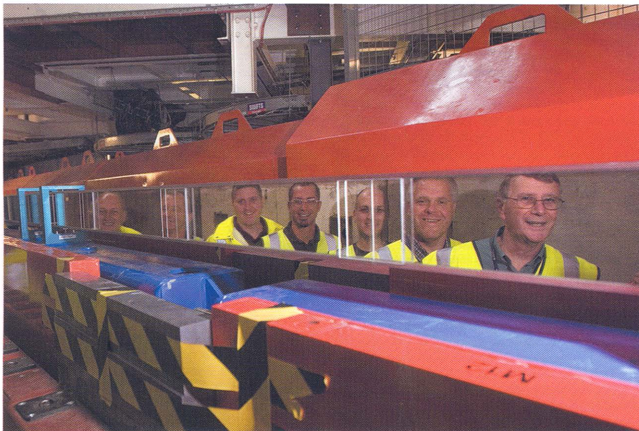
Figure 2. The new elliptic supermirror guide of the HRPD beam line at ISIS. The insert shows the flux increase relative to the original Nickel guide. (Picture courtesy of ISIS).
