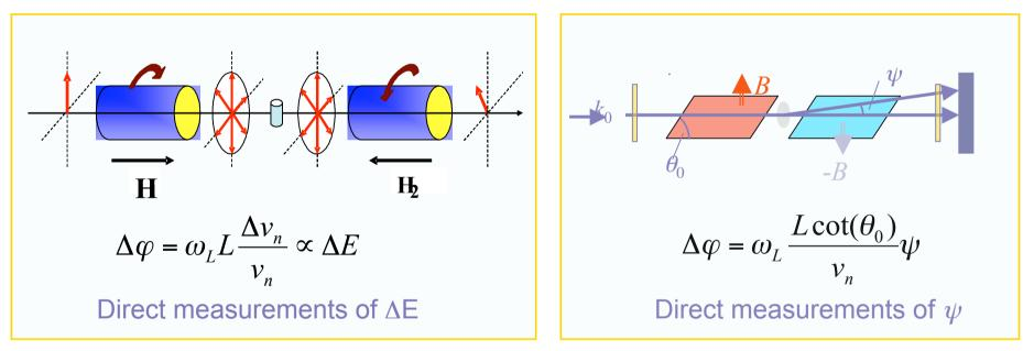
An extremely high energy (momentum) resolution that is not possible in conventional neutron spectroscopy (diffraction) because of intolerable intensity losses, become achievable.
