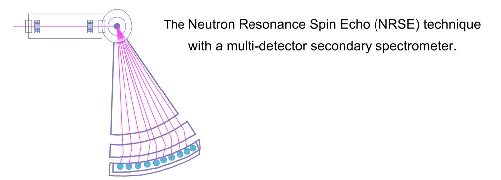
We will develop large solid angle NRSE coils allowing for the parallel data acquisition in a wide Q-range and thus resulting in a tremendous gain in the data acquisition rate.
