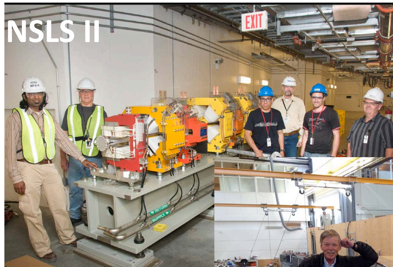
NSLS-II First Girder: 14-foot, 8-ton structure holding multiple magnets installed in the accelerator ring. June 15, 2010
