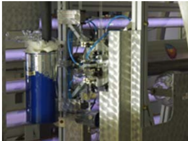
Fig J4: The world's best MEOP filling station for neutron scattering located at ILL, Grenoble (France). In this photo, we see the head of the non-magnetic piston used to compress the polarised gas. In the back, we also see the light emitted by the plasma of ^3\text{He} obtained by applying a discharge. The whole apparatus is about 2m diameter and 3m long. A very homogeneous magnetic field of 8 Gauss is applied in the whole system.
