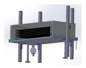
The demonstrator will incorporate a stack of 3 macro structured planes and 2 wire planes
