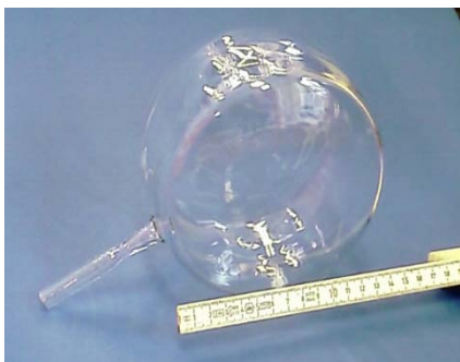
Figure 36: The largest in the world ^3\text{He} cell made of the GE180 glass manufactured in the FZJ.
