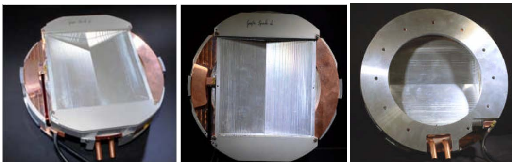
Figure 38: Assembly of a new large set of Pythagoras coils with central water cooling.
