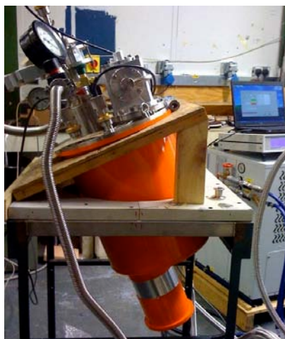
Figure 52: Top-loading cryogenerator at LLB. General view of the cryostat during testing at 20° tilt.
