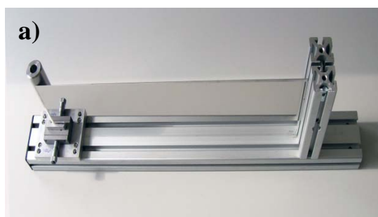
Figure 14: : a) Prototype of an adjustable focusing device using a mechanical bending mechanism. b) Defining parameters of the parabolic focusing device. The parameters to define the parabola are the rotation angle \alpha and the movement x .
