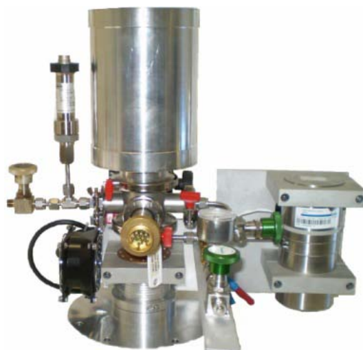
Figure 54: Pulse tube refrigerator for in-situ gas adsorption experiments.
